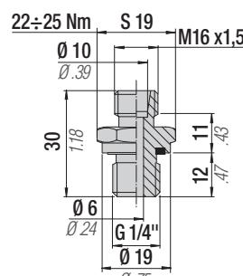
Raccordi di derivazione - Offtake connections - Anschlüsse zwischen schlauch und Zylinder/Kontrollarmatur - Raccords tuyau-cylindre/tableau - Racores manguera-cilindros/panel - Racord tubo-cilindro/painel
