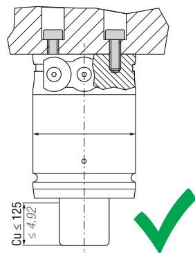
Installation with bottom fixing screws in upside down position.
