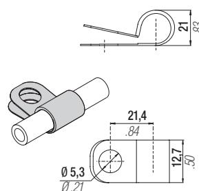
Raccordi tubo-cilindro/pannello - Hose-cylinder/panel connections - Anschlüsse zwischen schlauch und Zylinder/Kontrollarmatur - Raccords tuyau-cylindre/tableau - Racores manguera-cilindros/panel - Racord tubo-cilindro/painel
