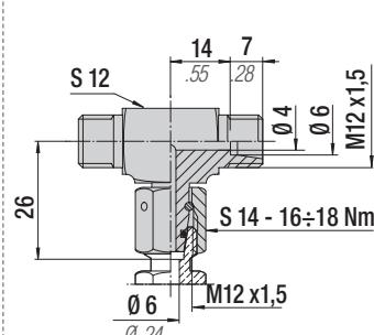
Raccordi tubo-tubo - Hose-hose connections - Anschlüsse zwischen Schlauch und Schlauch - Raccords tuyau-tuyau - Racores tubo-tubo - Racord tubo-tubo
