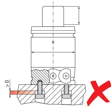
Installation NOT allowed due to incorrect screw length.
