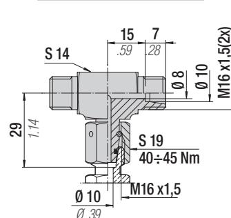
Raccordi tubo-tubo - Hose-hose connections - Anschlüsse zwischen Schlauch und Schlauch - Raccords tuyau-tuyau - Racores tubo-tubo - Racord tubo-tubo
