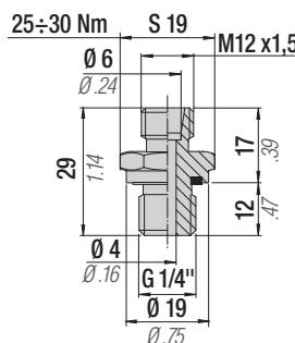
Raccordi di derivazione - Offtake connections - Anschlüsse zwischen Stutzen - Raccords de dérivation - Racores de derivación - Racord de derivação
