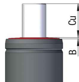
The secondary wiper don't reduce the nominal stroke of the cylinder.
