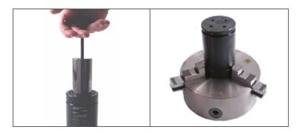
Extract the piston rod from the cylinder body and place it upside down in a self- centering holder.
