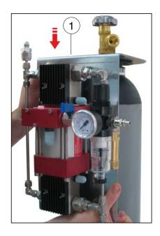
Position the support plate 1 with the mounted booster on the nitrogen bottle.
