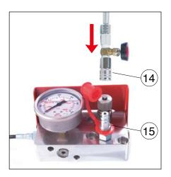
Connect the quick female connector (14) to the quick male connector (15) installed on the control panel.
